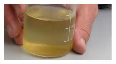
**Figure 18.** A sample of water containing iron
