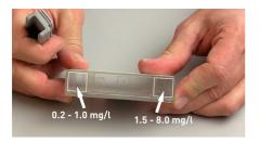
**Figure 3.** The three chambers of the comparator
