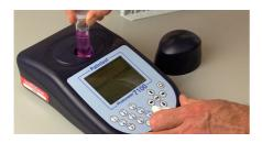
**Figure 15.** Inserting the test tube into the photometer
