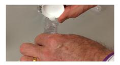
Figure 13. Adding the nitrate test tablet
