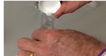
Figure 13. Adding the nitrate test tablet
