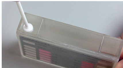
Figure 6. Crushing the tablet
