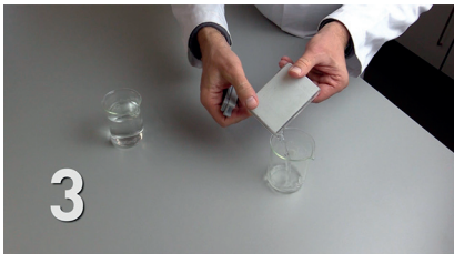
Figure 4. Rinsing out the comparator
