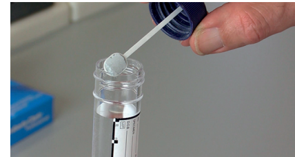
Figure 12. Adding the nitrate powder
