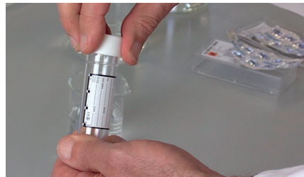
Figure 11. A screw top bottle for testing samples containing nitrate
