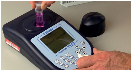
Figure 15. Inserting the test tube into the photometer
