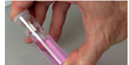
Figure 14. Adding the nitricol tablet will cause the colour to change
