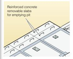
**Figure 15.** Handles can make removing the slab easier
