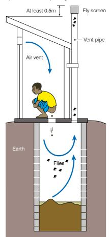
**Figure 10.** The design of the slab can direct the flow of air
