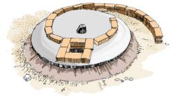
**Figure 23**. A round slab providing the foundation for part of the wall of the superstructure
