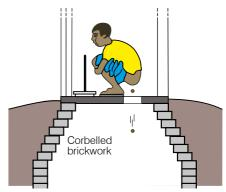
Figure 26. Corbelled brickwork lining
