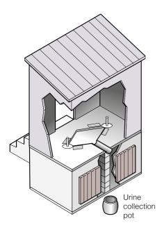
**Figure 8.** Urine diversion toilets require specific slab designs
