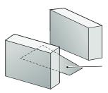
Tapered toilet drop hole in concrete slab
