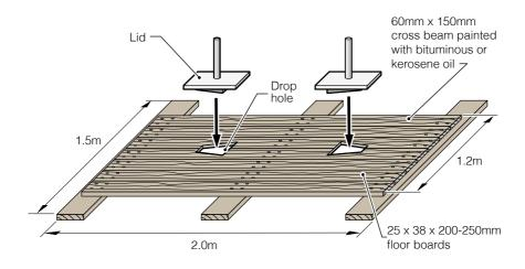
Figure 19. Slabs can be made of wood, but should be treated with preservatives
