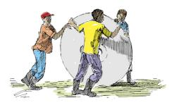
**Figure 6.** Circular slabs can be rolled into position, making them easier to move over short distances
